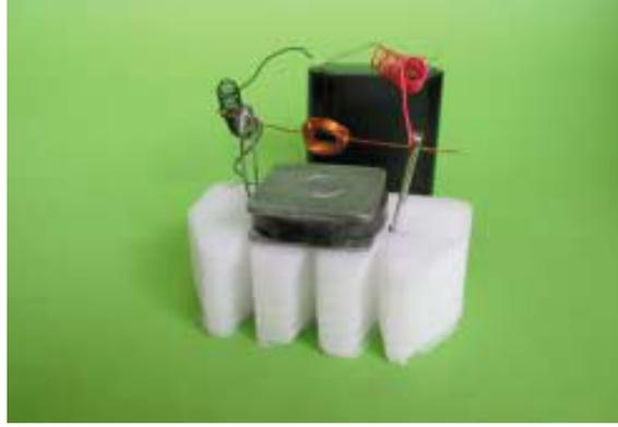
**Figure 1.** A simple electric motor circuit
